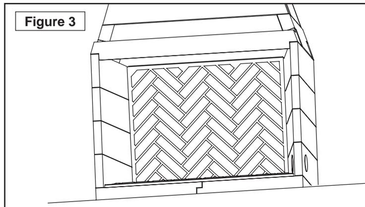
Apply mortar also along the bottom at the front side where the hearth meets. A placeholder will be required to retain rear wall in position while it is curing.
