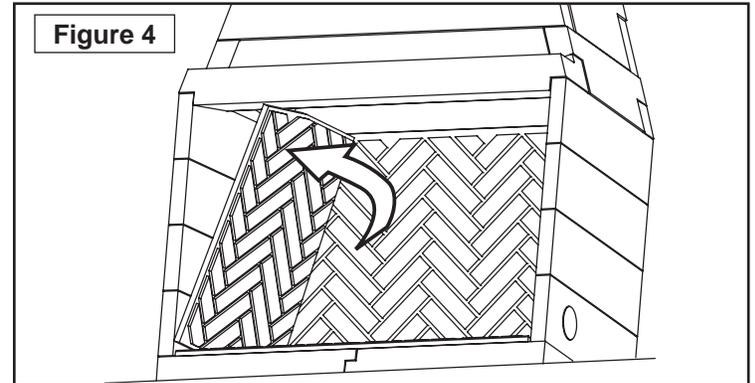
Gently tap the brick face with a rubber hammer to seat the side panel properly. Do not hit too hard or the panel may get damaged if it is still curing. Do not hit rear panel since there will be a void behind it and may cause damage. A placeholder will be required to maintain the side wall in place while the mortar cures.
